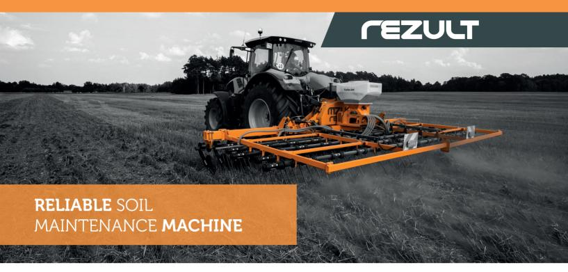
The REZULT straw rake marks a major advance in straw and stale seedbed management, and is the ideal tool to control black-grass and other weeds, cut slug activity and accelerate straw decomposition. By working at a shallow depth of 1-2 cm, the rake stimulates the faster emergence of weed seeds, preparing the field drilling.
